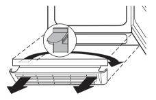
Close the freezer compartment door. Open the fridge compartment door and unscrew the retaining screw for the self-closing mechanism on the top of the freezer compartment door.
